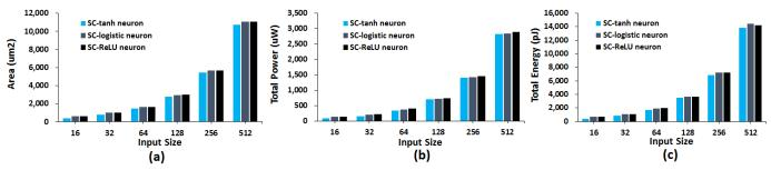
Fig. 6. Input size versus (a) area, (b) total power, and (c) total energy for the neuron designs using tanh, logistic and ReLU activation functions.
