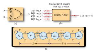
Fig. 3. Stochastic computing for neuron design: (a) XNOR gate for bipolar multiplication, (b) binary adder for average pooling, and (c) FSM-based tanh for stochastic inputs.
