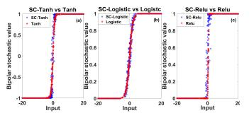
Fig. 4. The result comparison between the proposed SC neuron (bit stream m=1024) and the corresponding original software neuron: (a) SC-tanh vs Tanh, (b) SC-logistic vs Logistic, and (c) SC-ReLU vs ReLU.
