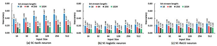
Fig. 5. Input size versus absolute inaccuracy under different bit stream lengths for (a) SC-tanh neuron, (b) SC-logistic neuron, and (c) SC-ReLU neuron.
